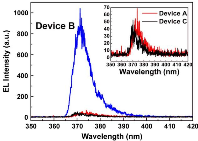
Fig. 2. EL spectra of the ZnO-based MIS LED devices of A, B, and C when applied with a forward bias of 3 V. The inset shows the same EL spectra of devices A and C in a smaller range.
