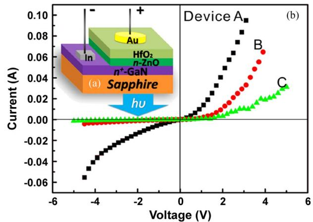
Fig. 1. (a) Schematic diagram of the Au/HfO<sub>2</sub>/n-ZnO MIS structure on an n<sup>+</sup>-GaN/sapphire substrate. (b) Current–voltage characteristics of the ZnO-based MIS LED devices of A, B, and C.
