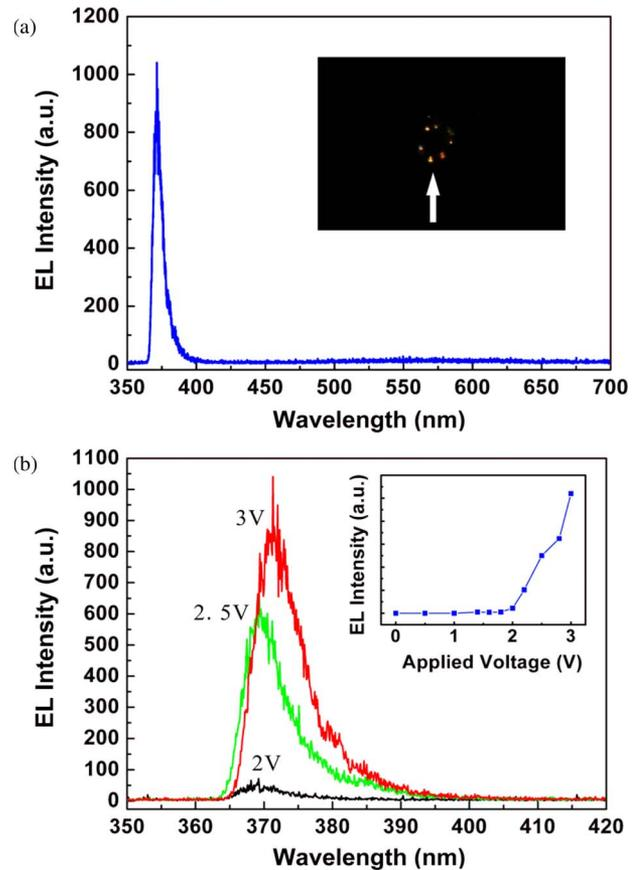
Fig. 3. (a) RT EL spectrum of the ZnO-based MIS LED with  $\sim 50\text{-nm}$ -thick  $\text{HfO}_2$  layer applied with a forward bias of 3 V. The inset shows the lighting image of the ZnO-based MIS LED device. (b) RT EL spectra of the ZnO-based MIS LED device under various forward bias voltages of 2, 2.5, and 3 V. The inset shows the plot of EL intensity versus forward bias fixing the emission wavelength at 371 nm.
