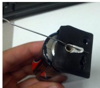
7. To hold the bent paperclips in place stretch both rubber bands around the base of the battery case.
