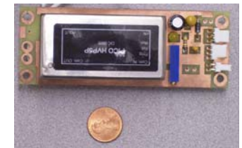
4 Miniaturized Gate Controller circuit (left) and High Voltage Supply circuit (right) produced by PCB router
